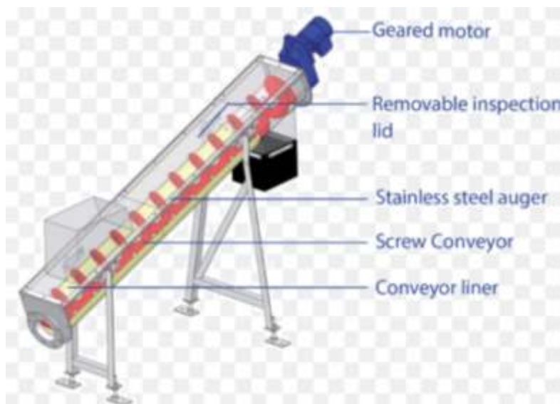
Figure 2.6: Labelled incline screw conveyor (KWS, 2016)
