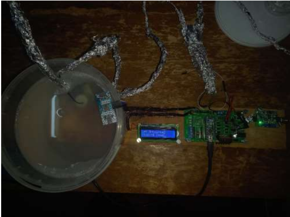
Figure 5.14: an image showing the LCD display when pH was less than 9
