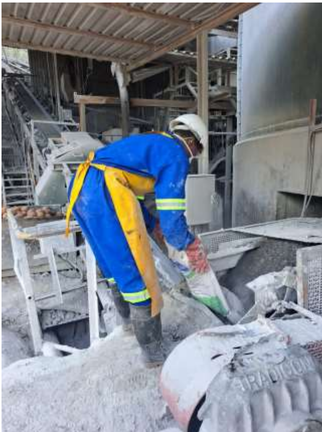
Figure 1.4: A picture of an operator putting lime onto a moving conveyor
