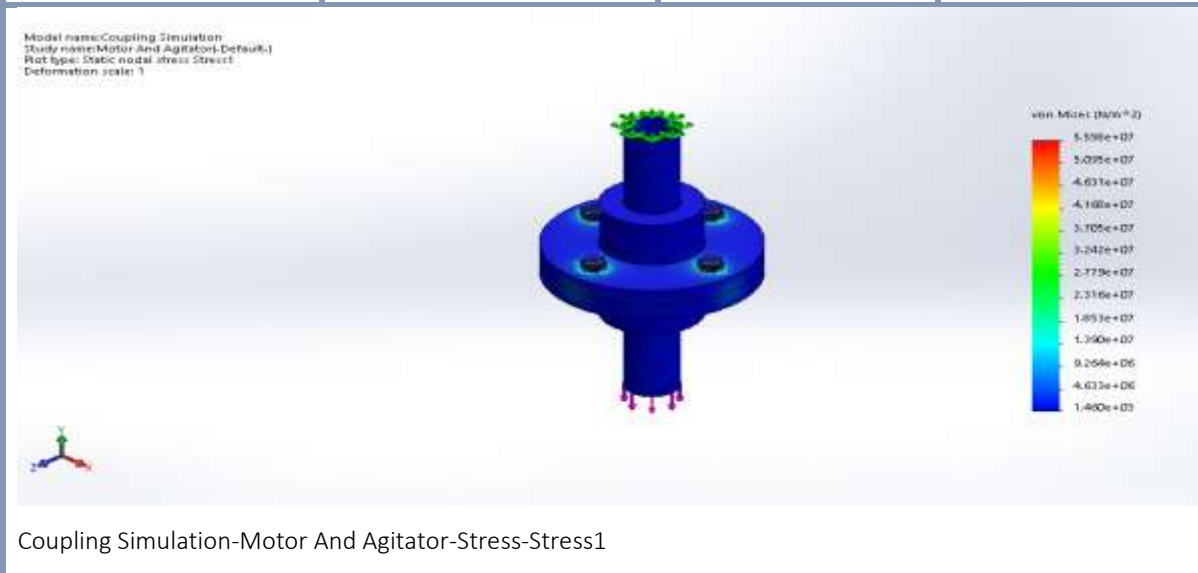
Figure 5.8- Von Mises stress simulation results
