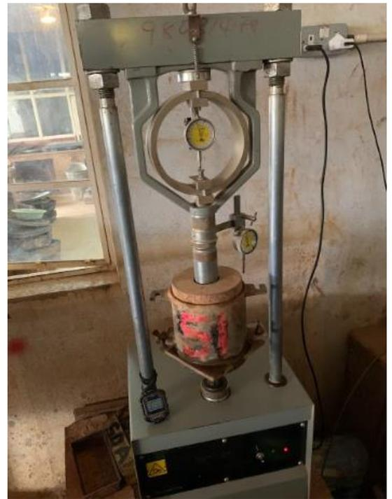
The CBR machine used for strength determination of both the dry and soaked compacted samples, treated and untreated
