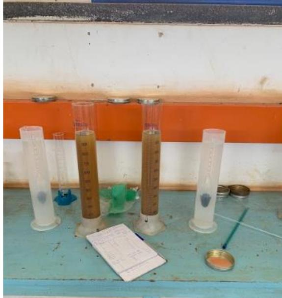
*Figure 3.3: Set up of apparatus used for hydrometer analysis test.*
