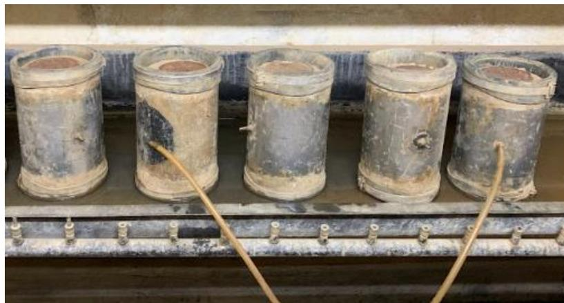
*Figure 3.8: Saturation stage where samples were left to soak in a water bath.*
