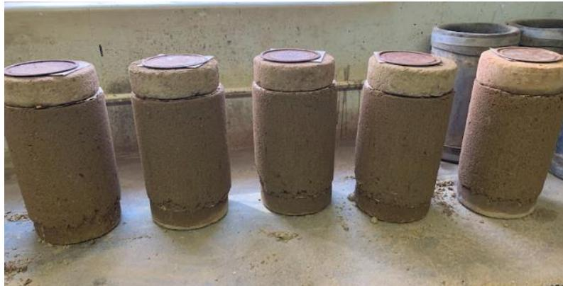
*Figure 3.7: Samples prepared for triaxial shear test.*
