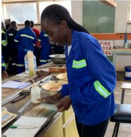
*Figure 3.5: Plastic limit test.*
