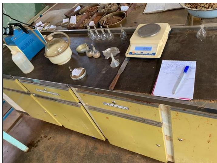
*Figure 3.4: Apparatus used for specific gravity determination.*
