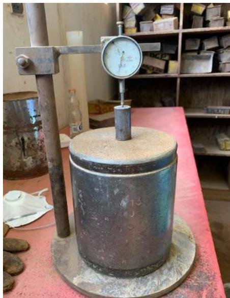
*Figure 3.6: Dial gauge used to measure the height of specimen.*
