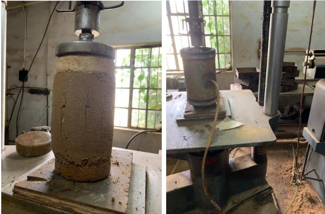
*Figure 3.9: Triaxial test compression stage*
