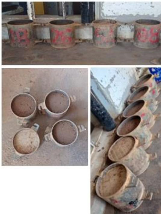
Control and treated samples compacted and left to cure for 7 and 28 days.
