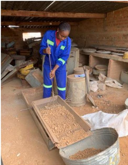
Screening the sample (separating fine material from coarse) in preparation for backmixing and testing
