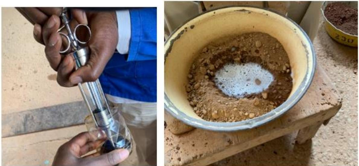
*Figure 3.10: Measurement of 1ml of EarthZyme road stabiliser and its addition to water in the soil sample during compaction.*
