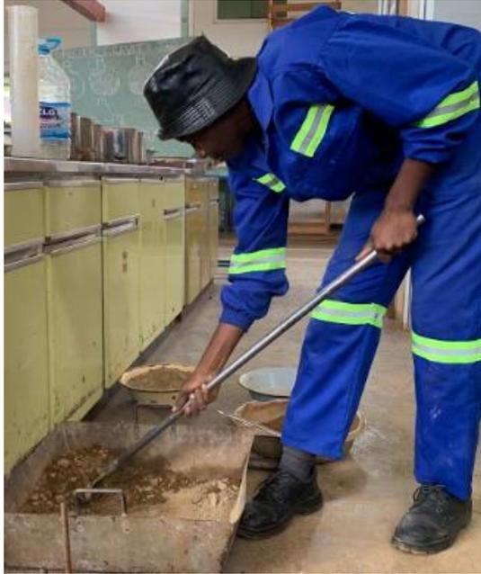
Preparation of sample for compaction.
